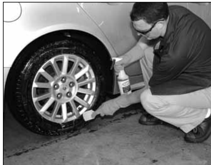
Agitate the Cleaner on the tire with a stiff bristled brush to remove embedded road film.
