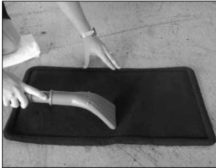
Thoroughly vacuum and towel dry the fabric surfaces to be dyed.
