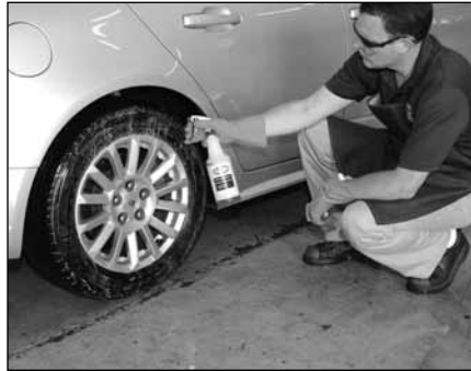
Spray both the wheel and tire with a non-acid Wheel Cleaner, and allow it to dwell for one minute.
