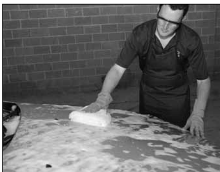
Since Car Soaps are pH balanced (contain no harsh alkalis), agitation is required to break the bond between the soil and the vehicle surface.
