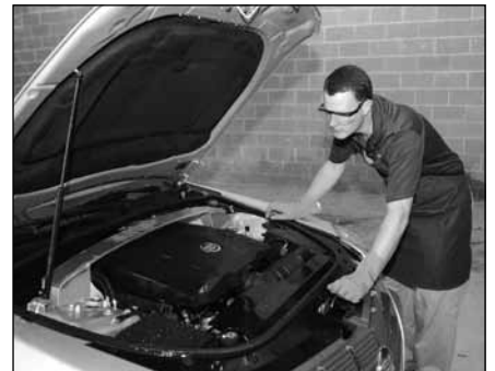
Examine your work. If any dirt or grease remains, re-apply the Cleaner/Degreaser and re-rinse.
