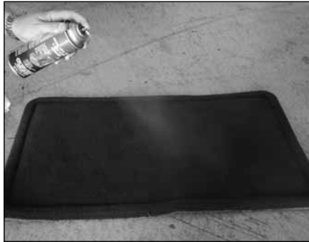
Spray a light coating of dye directly on the fabric.
