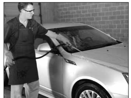
Rinse the vehicle from the top down, using low pressure.
