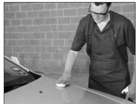
Gently rub the Clay Bar over the lubricated surface, working lengthwise with the panel.
