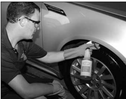
Spray the wheel wells with a solvent-based dressing.
