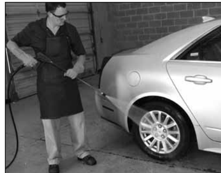
Thoroughly pressure rinse both the wheel and tire.
