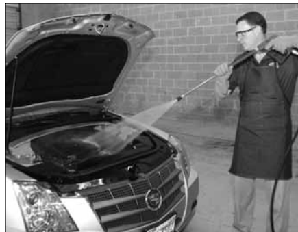
Thoroughly rinse the engine following a consistent pattern. Stand at different angles to ensure hard-to-reach areas are completely clean. Don't saturate engine electronics.
