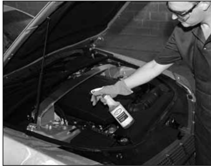
Spray the entire engine with a water based dressing, using a consistent pattern to ensure even coverage.
