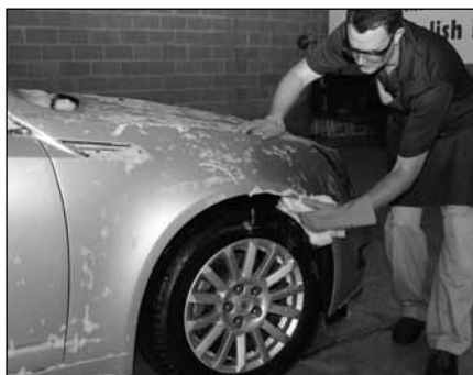
Be sure to "mitt out" the wheel wells (using a separate mitt than the one used to agitate the soap solution on the paint).
