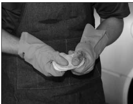
Knead the Clay Bar when its face become "saturated" (there is no longer any resistance as you rub the bar on the paint).
