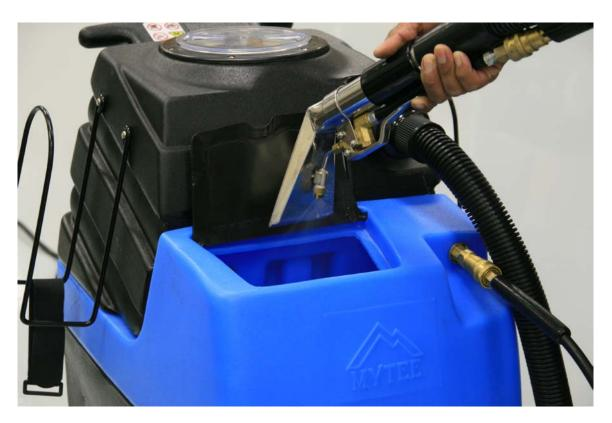
3. Turn on Pump. Put detail wand into solution tank and pull the trigger on the valve assembly to spray solution back into tank. A nylon zip-tie works good to keep the solution spraying. Allow pump to recirculate solution for 10-15 minutes.
