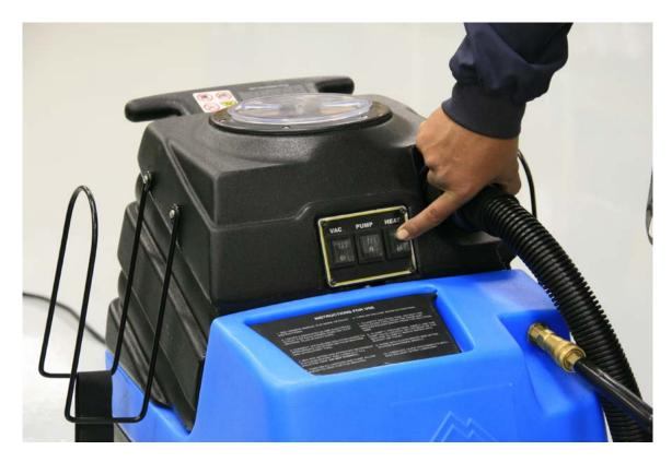
2. Turn on Heater to preheat extractor to operating temperature. Depending on the heater setup this can take anywhere from 4-20 minutes.
