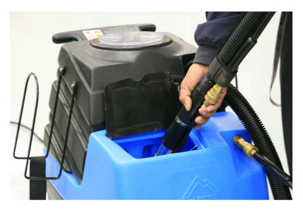
4. Turn on Vacuum. Using the detail wand, vacuum out contents of solution tank.
