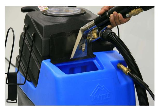
7. Turn on Pump. Put detail wand into solution tank and pull the trigger on the valve assembly to spray solution back into tank. Allow pump to recirculate fresh water for 1-2 minutes.
